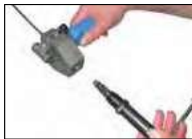
Step 3 Insert the punch and ram
