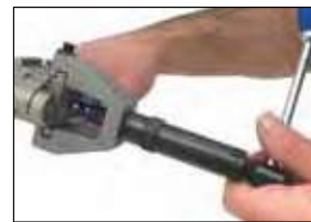
Step 4 Turn T-Bar to create the flare
