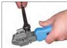
Step 2 Tighten the clamping nut
