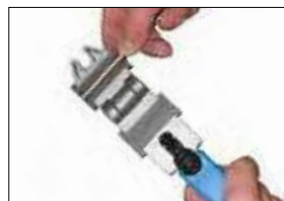
Step 1 Place the pipe in the die
