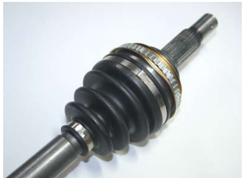
CV Boot Clamps used on constant velocity joint
